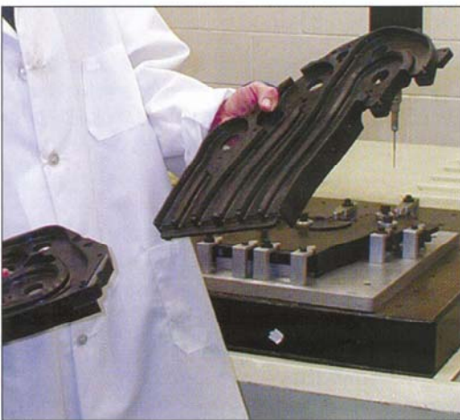
Cartridge guides molded by Parkway Products for General Dynamics Armament and Technical Products division display complex contours, vertical walls and varying thicknesses — all produced successfully and efficiently by compression molding.
