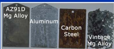
CORROSION AFTER 10-DAY SALT SPRAY TEST
